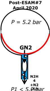
Nitrogen continues to permeates membrane to form gas bubbles as N2H4 is already fully saturated
