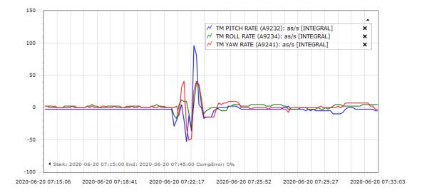
Use of thrusters causes significant loss in RCS pressure at each actuation
