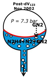
$P1 = 7.3 \, bar$ **Pressure drop forces** some N2 out of solution, due to super-saturation, to form GN2 bubbles
