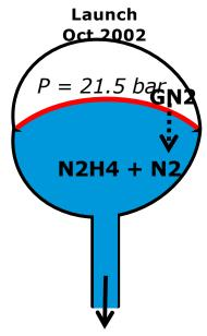
$P1 = 21.5 \, bar$ Nitrogen permeates membrane, gets absorbed into solution within N2H4 and then expelled through thrusters
