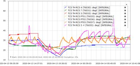
2<sup>nd</sup> SEU? isolates Propellant System Heater B, about 2 hours later
