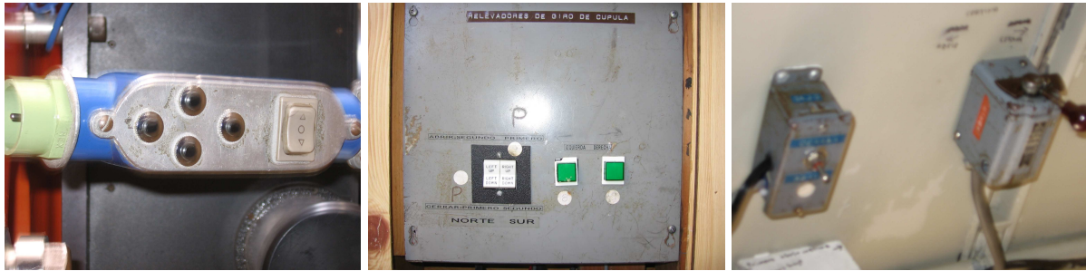
Figure 9: Dome/telescope paddle (left), dome controls (green buttons, center), mirror cover controls (white buttons, center) and the dome opening controls (right).
