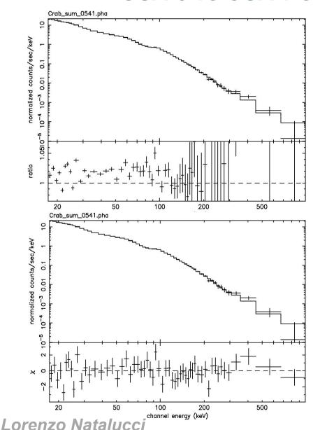
Rev.541 OSA-8 spectrum fit by OSA-7 ARF built on the same revolution
