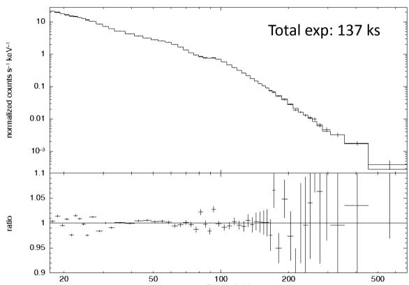
Fit of average Crab spectrum measured on an extended period (~2.5 years, source on-axis)
