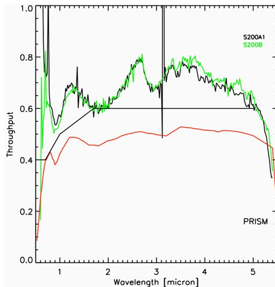
**Figure 2: End-to-end instrument throughput for the NIRSpec PRISM, estimated using the calibrated lamp spectra for the CLS lamp FFB as reference. Spectra for two NIRSpec slits are plotted. The lower red curve indicates the expected throughput based on component-level measurements. The horizontal black line marks the requirement NSFR-042 listed in Appendix A.**
