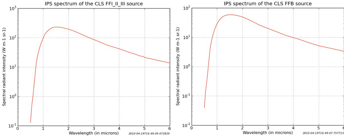
**Figure 1:** Output spectra for CLS lamps FF1-3 (left) and FFB (right), as measured by MSSL.
