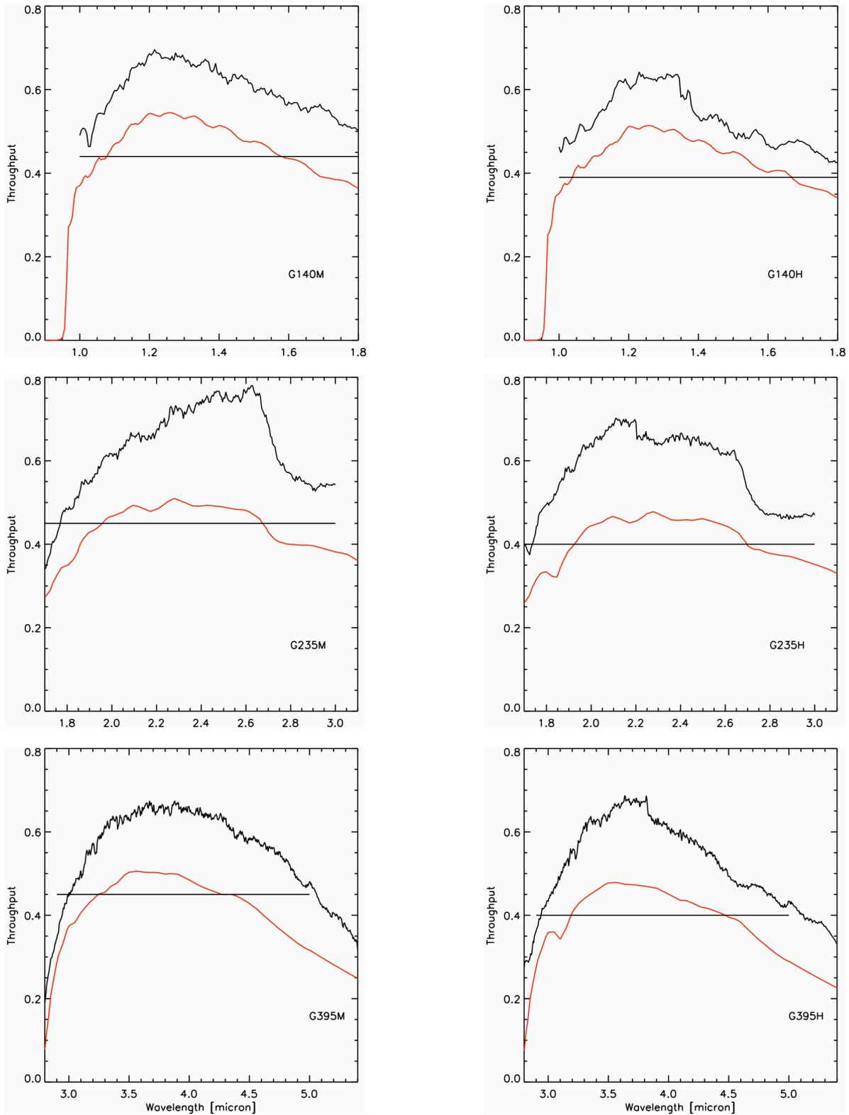
**Figure 3: End-to-end instrument throughput for the six NIRSpec gratings (black curves), estimated using the calibrated lamp spectra for CLS lamps FF1, FF2, and FF3 as reference. For comparison, the expected throughput based on component-level measurements is also shown (red curves). The black horizontal lines denote the requirements listed in Appendix A.**
