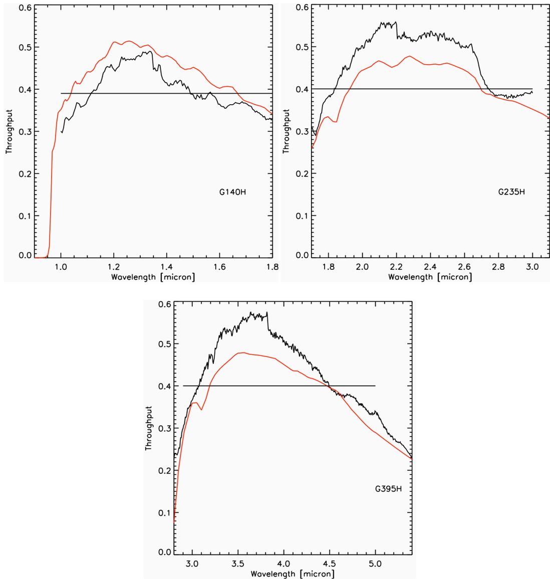
**Figure 4: End-to-end instrument throughput for the three high-resolution NIRSPEC gratings (black curves), estimated using data from the *PREP-CLS-XCAL-D* test procedure, and the calibrated lamp spectrum *sourceCLS\_NAKED.src* as reference. For comparison, the expected throughput based on component-level measurements is also shown (red curves).**
