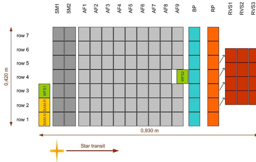
FIG. 1.8 – Plan focal du satellite Gaia, EADS Astrium 2006
