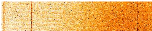
FIGURE 14: LR-R spectrum of the He lamps observed through the 2” slit + B filter and 3600 sec exposure time. Three lines are visible, two in the blue (left) and one unexpected in the red (right).
