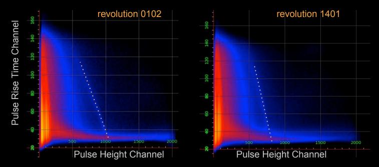
Irradiation of detector changes lifetime of charge carriers, decreasing pulse height, causing pulse height drift The reconstruction must be time-dependent
