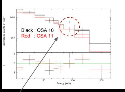
excess at 100 keV was mildly significant, but strongly affected slope! spectrum of a magnetar provided Lin Lin, 2 Ms observations.
