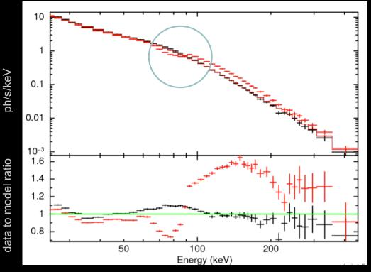
broken powerlaw, only normalization fitted to OSA11, break at 100 keV, LE slope 2.1 (SPI), HE slope 2.21 (all-mission fit ISGRI). Revolution 839 of Crab calibration
