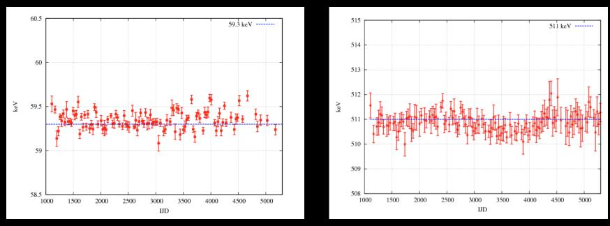
Line positions fitted in the OSA11 background spectra, averaged over one month. Unstable fit removed.
