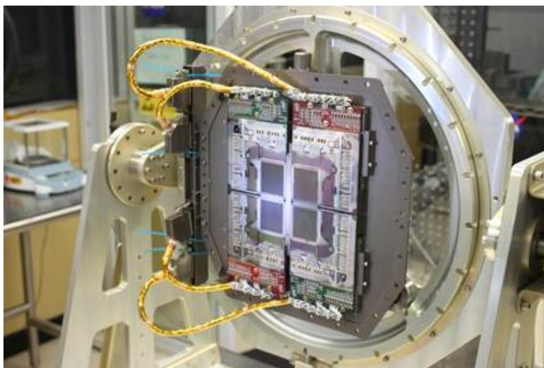
Figure 5. Image of the new MSA (without the full enclosure) to be installed in NIRSpec following the ISIM CV2 test campaign. Credit NASA.
