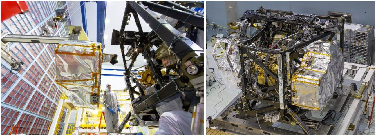
Figure 4. Left: NIRSpec on the Horizontal Integration Tool during installation to ISIM. Right: Image of the fully assembled ISIM structure, with NIRSpec visible on the right. Credit NASA.
