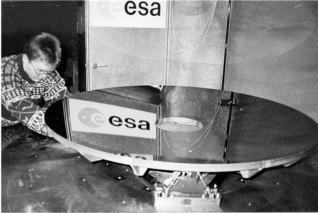
Figure 4.4: FIRST 1.35 m Silicon Carbide reflector, demonstration model made of nine brazed segments (courtesy MMS).
