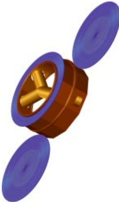
Figure 4-3 Artist's concept of the LISA spacecraft attached to the solar-electric propulsion module. The ion-engine is mounted at an angle to the wall of the main cylinder of the propulsion module in order to thrust through the combined center of mass. The ion engine requires power from two deployable solar arrays which are gimballed to allow for tracking the Sun. Not shown is a cover over the top of the cylinder that prevents sunlight from striking the Y-shaped payload enclosure.
