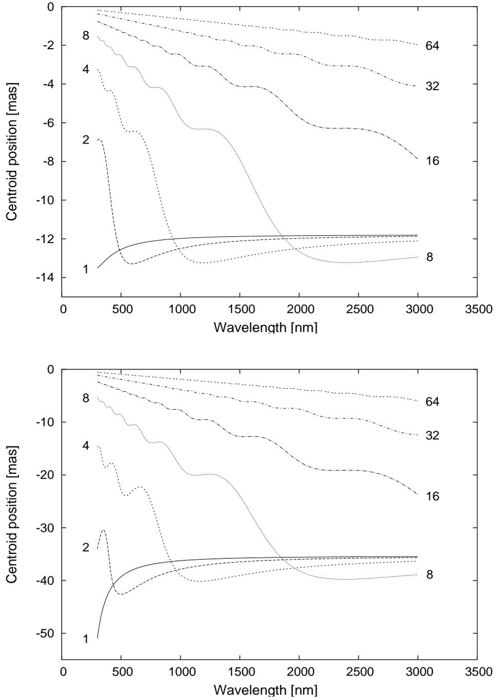
FIGURE 2: Examples of the behaviour of the monochromatic centroid defined by the truncated mean (21) for the WFE cases shown in Fig. 1. The upper panel is for the WFE shown as a solid curve in Fig. 1; the lower panel corresponds to the dashed curve in Fig. 1. The curves are labelled by the truncation width  $t$  expressed in pixels (1 pixel = 44.2 mas). A realistic centroid definition for Gaia will have  $t \simeq 2$  pixels.
