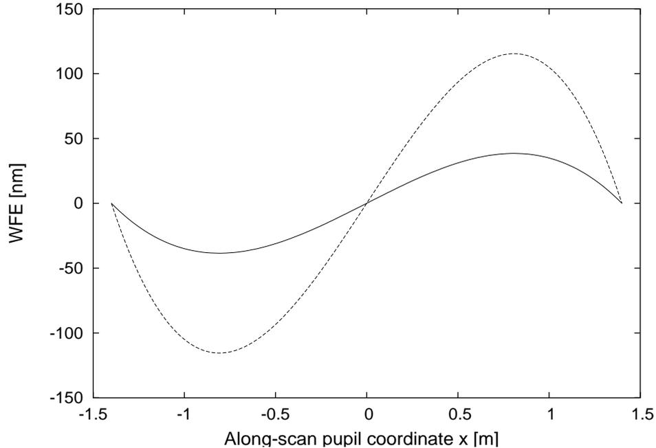
FIGURE 1: Assumed WFE for the two test cases with results in Fig. 2. The solid curve is for (24) with  $c = 100$  nm, the dashed curve is for  $c = 300$  nm. The mean tilt is, respectively, 11.79 mas and 35.36 mas. The RMS wavefront error after removing the tilt is 15.2 nm and 45.4 nm. Other optical parameters are:  $D = 1.4$  m, focal length = 46.7 m, along-scan pixel size =  $10 \mu\text{m}$ .
