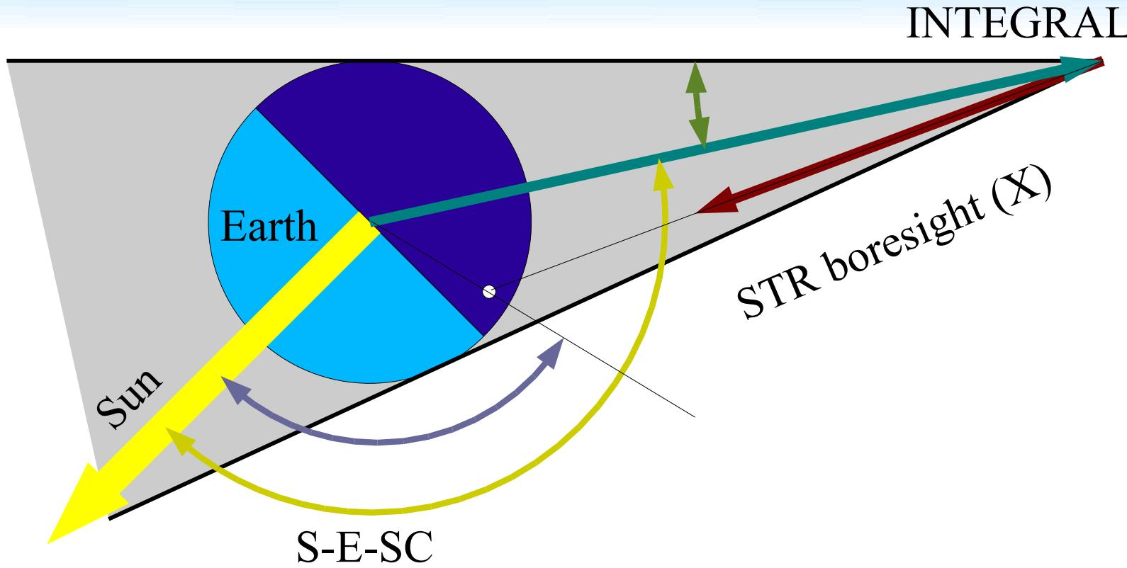
**The Sun-Earth-Location Angle (S-E-Loc): Measure for illumination of the location to which the STR points**
